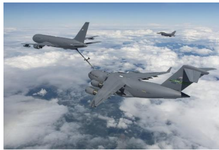
A KC-46 tanker (top) refuels a C-17 transport in mid-air
